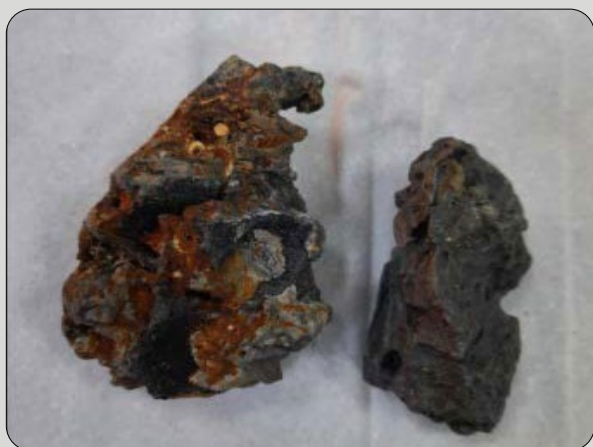
E-221-004 Hardened scale material found at condenser outlet boot
