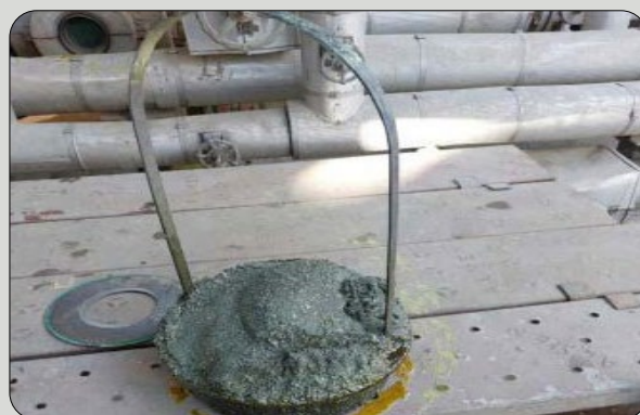
Strainer of E-221-005 is shown: E-221-0005 Sultrap strainer material 29/11/21
